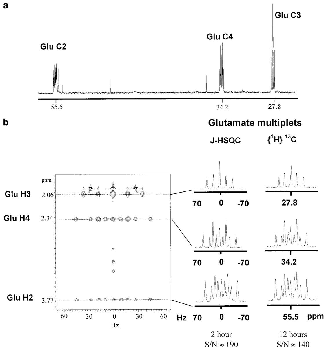
**FIG. 2.** (a)  $\{^1\text{H}\}^{13}\text{C}$  NMR spectrum and (b) J-HSQC spectrum collected at 14.1 T of an extract of a mouse heart perfused to steady state with a mixture of  $[2\text{-}^{13}\text{C}]$ acetate and  $[1,2\text{-}^{13}\text{C}_2]$ acetate. The projection of the J-HSQC and the  $\{^1\text{H}\}^{13}\text{C}$  spectrum give the same multiplet data. Note the loss of isotopic shift in the J-HSQC spectra.
