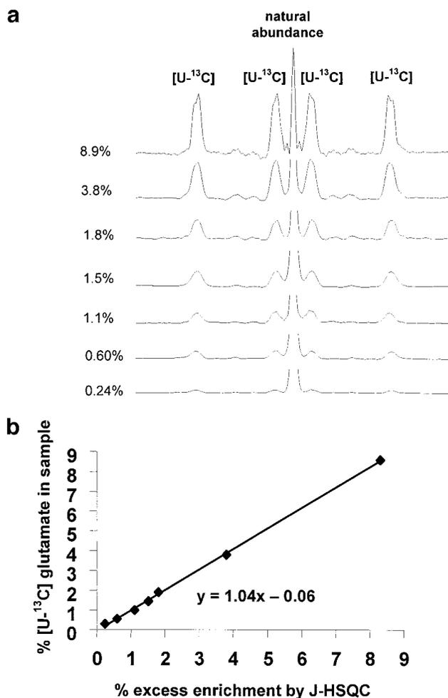
**FIG. 4.** (a) J-HSQC spectra of glutamate containing various amounts of added  $[U\text{-}^{13}\text{C}]\text{glutamate}$ . Total glutamate was 150 mM. (b) Plot of known chemical excess enrichment of  $[U\text{-}^{13}\text{C}_5]\text{glutamate}$  as measured analytically versus excess enrichment as measured by J-HSQC. The latter values were obtained by measurement of quartet versus singlet resonance areas in each spectrum.
