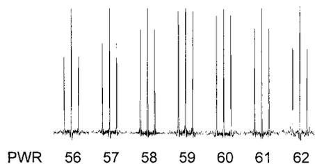
**FIG. 1.** The effect of imperfect refocusing pulses on the multiplet intensities of the 2:1  $[1,2\text{-}^{13}\text{C}_2]:[2\text{-}^{13}\text{C}]$ acetate standard. The appropriate RF power was calculated to be 59 dB by the pulse-shaping software.
